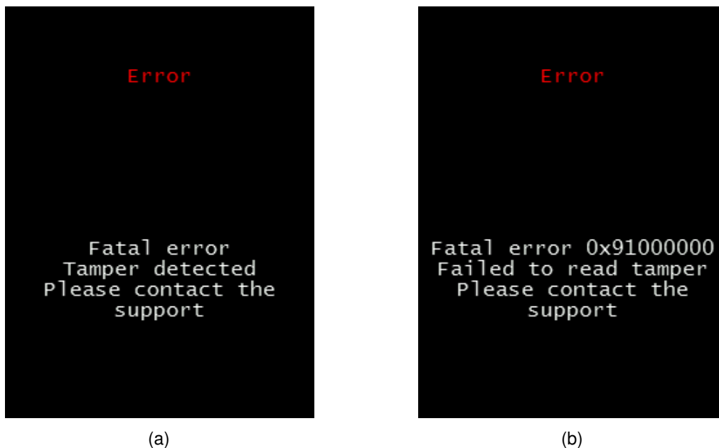
Figure 4.1: Display content in event of tamper. (a) After tamper condition has been restored. (b) With tamper condition still active.
