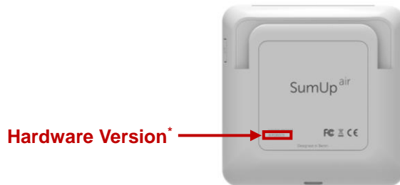
Figure 2 – Product Hardware Version Identification
