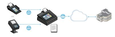
A **PAYMENT SYSTEM** includes the entire process for accepting card payments. Also called the cardholder data environment (CDE), your payment system may include a payment terminal, an electronic cash register, other devices or systems connected to a payment terminal (for example, Wi-Fi for connectivity or a PC used for inventory), and the connections out to a merchant bank. It is important to use only secure payment terminals and solutions to support your payment system.
