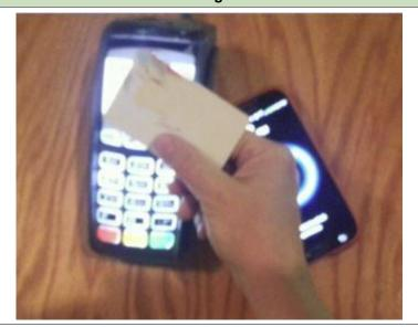
In an NFC attack, an NFC reader (in this case a smartphone) is placed between the terminal and the customer to capture the card data during a tap transaction.
